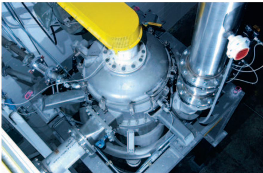
The CGS 71 fluidized-bed jet mill with stainless steel contact parts provides ultrafine grinding and tight particle-size control for reducing materials with sanitary requirements.
